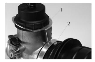
e) Only one rubber gasket is allowed to be used in the carburetor cap.
