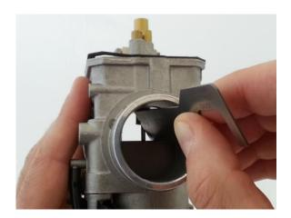
d) The position of the cap of the carburetor must be fixed by means of the fixation plate (pos. 1 see illustration below, ROTAX part no. 251 790).
